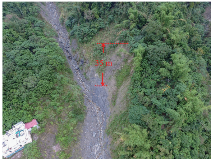
Fig. 4. The thick colluvial deposit observed at the toe of the slope at location 1.
