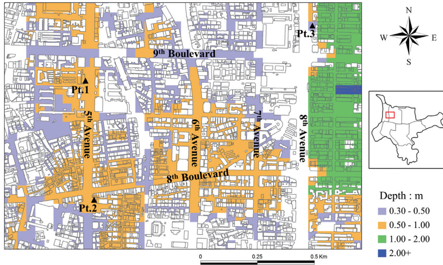
Fig. 13. Local simulated flood areas of Typhoon Nari with building blockage and storage effect (setting C).
