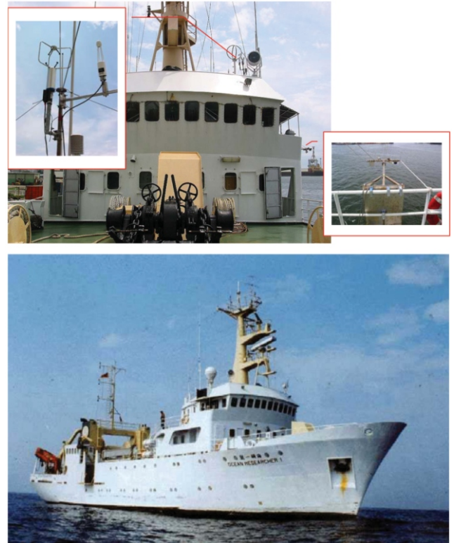
Fig. 2. Appearance of R/V OR1 and its equipped instruments, includes Eddy Covariance System (ECS), 3-D ultrasonic anemometer (81000, Young, USA) and an open path infrared hygrometer/ \text{CO}_2 sensor (7500, LICOR, USA), Eppley Pyranometer (PSP, EPLAB, USA) and an Eppley Pyrgeometer (PIR, EPLAB, USA).
