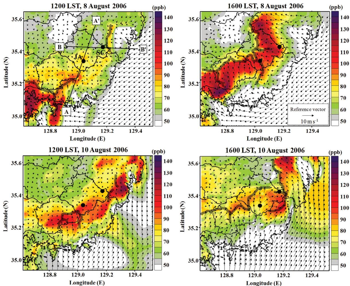
Fig. 3. Horizontal distributions of the simulated  $O_3$  concentrations (ppb) and wind vectors ( $m s^{-1}$ ) at 1200 and 1600 LST during the episodic days (8 and 10 August 2006). The thick lines indicate the wind convergence zones. A - A' and B - B' denote the vertical cross-section lines.
